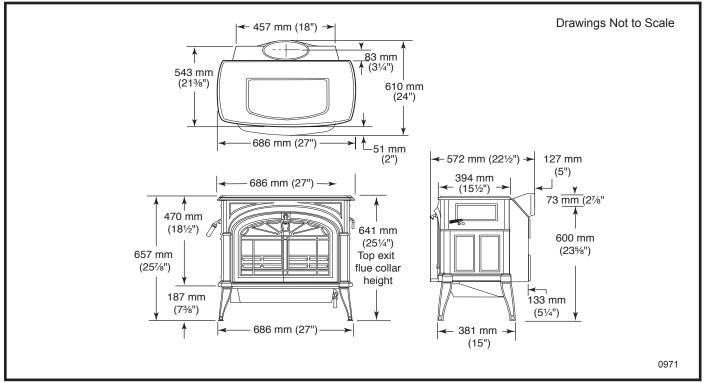
Fig. 1 Encore MF dimensions.
